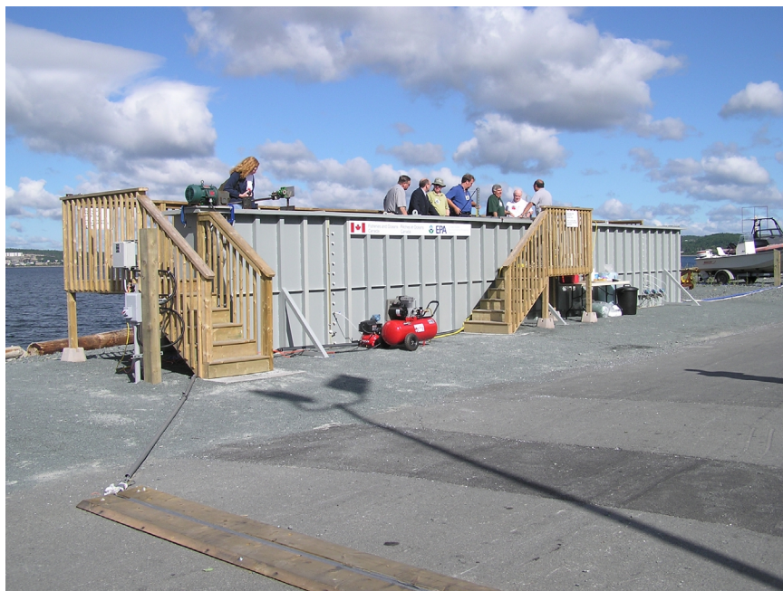
FIGURE 3-12 Photo of the EPA/DFO wave tank at BIO, Halifax, NS, Canada. SOURCE: K. Lee, Fisheries and Oceans Canada, Centre for Offshore Oil and Gas Environmental Research.
